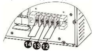
Diagram 2: 6KRT(L)/10KRT(L) Input/Output Terminal
