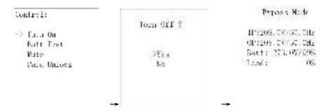
NOTE: You may simply turn off UPS by pressing "OFF/ESC" button in home page. It's not necessary to enter control menu to turn off the UPS.
