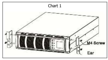
Step 2: Lift the UPS module and slide it into rack enclosure. Attach the UPS module to the rack with screws, nuts and washers (user-provided) through its mounting ears and into the rack rails. Please refer to chart 2.
