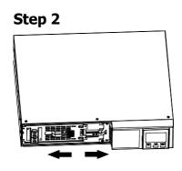
Disconnect battery wires.
