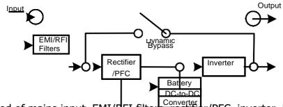
The UPS is composed of mains input, EMI/RFI filters, rectifier/PFC, inverter, battery charger, DC-to-DC converter, battery, dynamic by Battery and UPS output.
