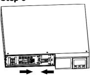
Re-connect the battery wires.
