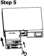
After replacing the batteries, put the battery box back to original location and screw it tightly.
