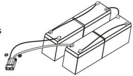
Step 4: Cover the other side of plastic shell as below chart. Then, battery kit is assembly well.
