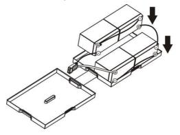
**6-battery kit** Step 1: Remove adhesive tapes.
