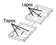
Step 3: Put assembled battery packs on one side of plastic shells as below chart.
