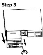
Pull out the battery box by removing two screws on the front panel.
