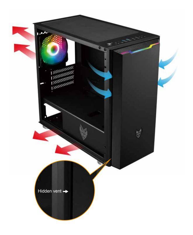
High flexibility for fan and water cooling support. Install any fan or water cooling systems you want. The case supports up to  $5 \times 120$ mm fans or  $2 \times 240$ mm radiators.
