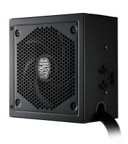
The MasterWatt is a 80 Plus Bronze Power supply with an innovative semi-fanless mode. Under 15% load, the MasterWatt fan remains idle, offering zero dBA. When demand for power increases, a gradual fan curve provides measured cooling with little to no noise at any output level. Dual forward / DC-to-DC topology are employed to keep the voltage stable in all conditions. For increased performance, MasterWatt is equipped with 16 AWG power cables, which reduce resistance thereby increasing efficiency.
