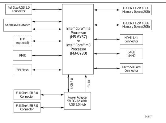
Figure 3. Block Diagram
