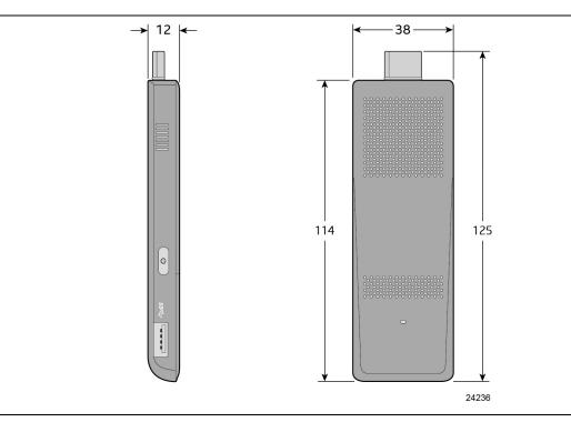
Figure 10. Intel Compute Stick Dimensions
