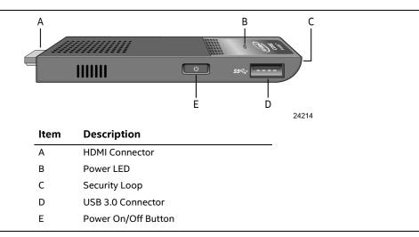
Figure 1. Left-Side View of Intel Compute Stick
