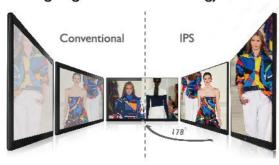
With IPS (In-Plane Switching) Technology, you see accurate color and image reproduction from any angle. An expansive 178° viewing angle is great for work and for reviewing on-screen with multiple people in the room.
