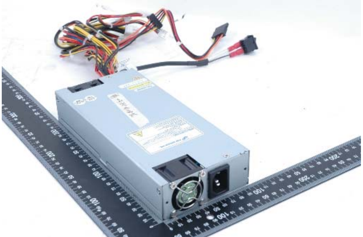
Model FSPxxx-701UH (Provided one flexible cord (near output side) for switch used, construction C)
