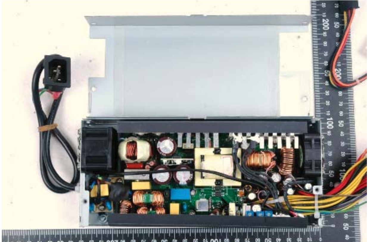
Model FSPxxx-701UH (Provided one flexible cord (near output side) for switch used, construction C)
