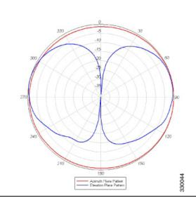
**Azimuth and Elevation Plane Patterns for 5 GHz**
