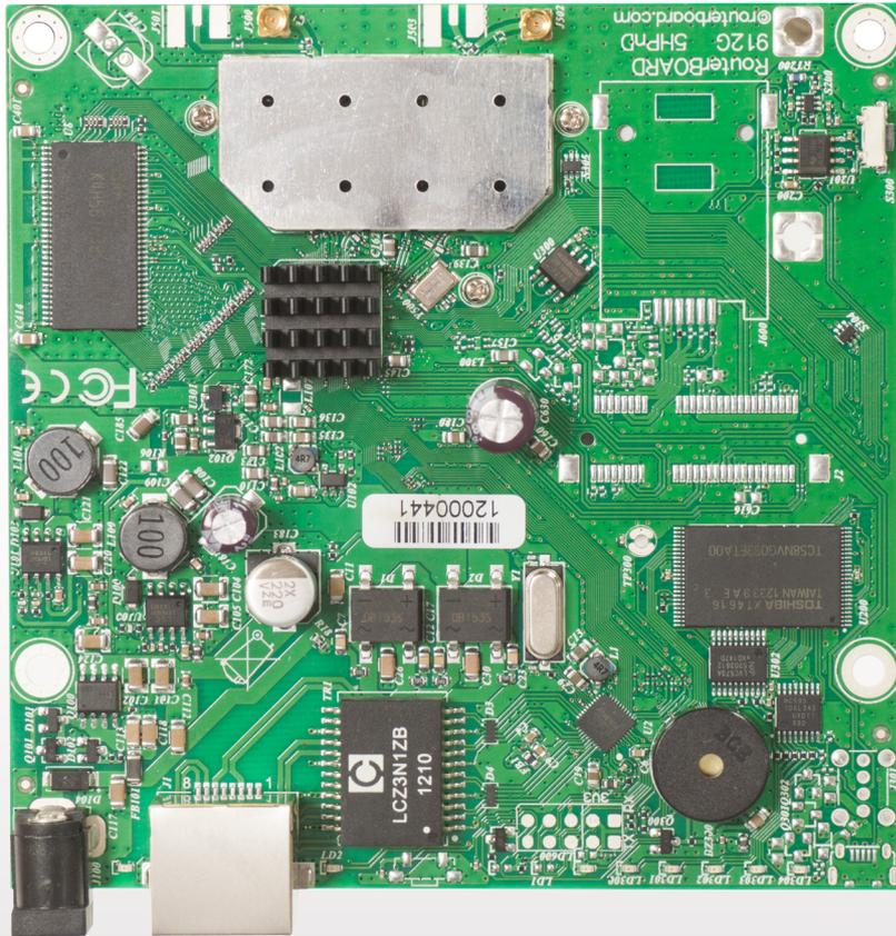
The RB911 is a small wireless router with an integrated high power wireless card. Both 2GHz and 5GHz models are available. The Gigabit port helps to utilize the full potential of 802.11n wireless speeds.
