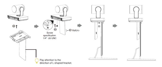
Choose the following installation method when the thickness of the TV is between 46 mm and 146 mm.
