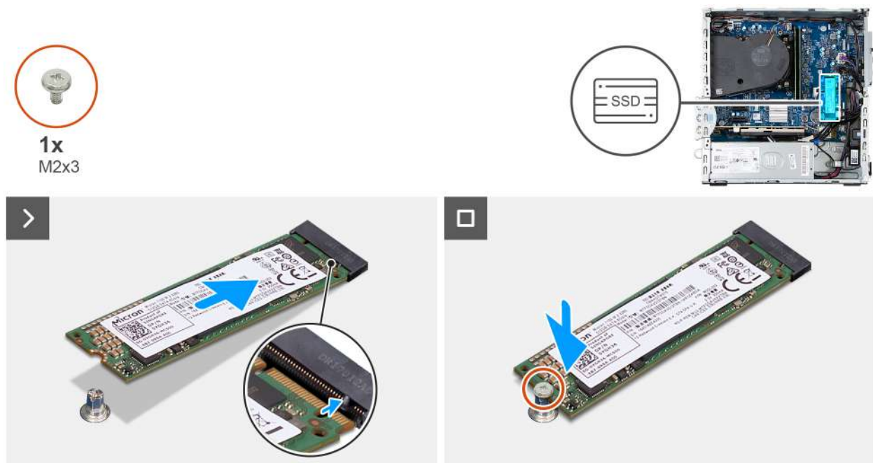
Figure 25. Installing the M.2 2280 solid state drive
