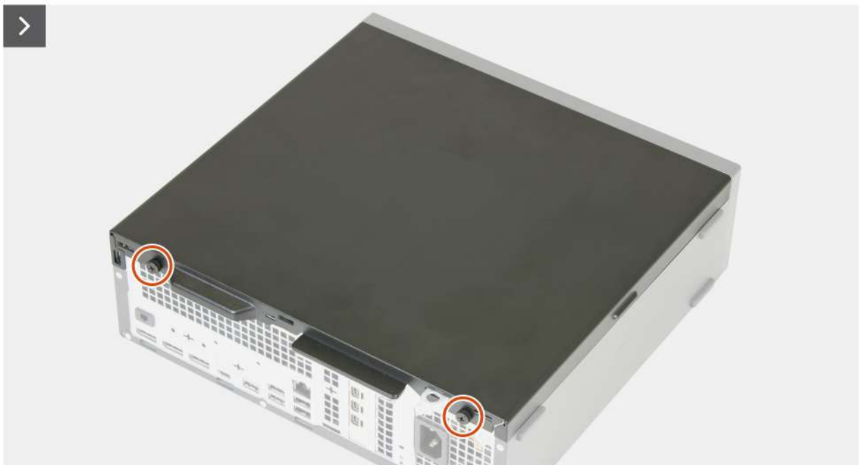
Figure 6. Removing the side cover
