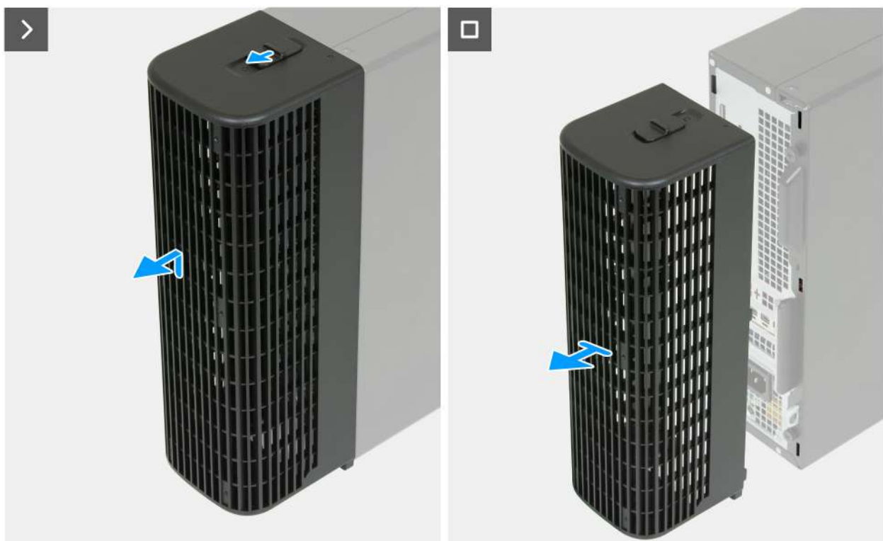
Figure 4. Removing the cable cover
