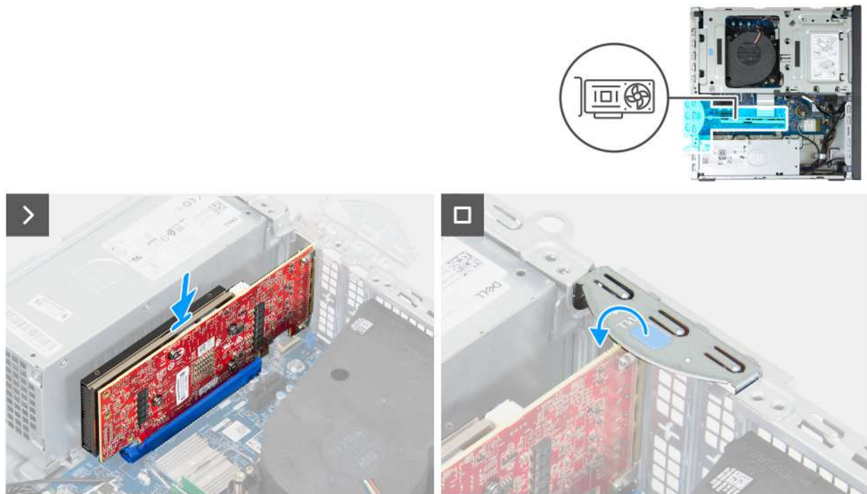
Figure 28. Installing the graphics card
