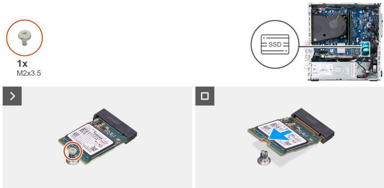
Figure 22. Removing the M.2 2230 solid state drive
