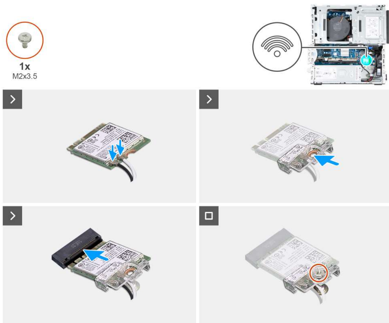
Figure 30. Installing the wireless card
