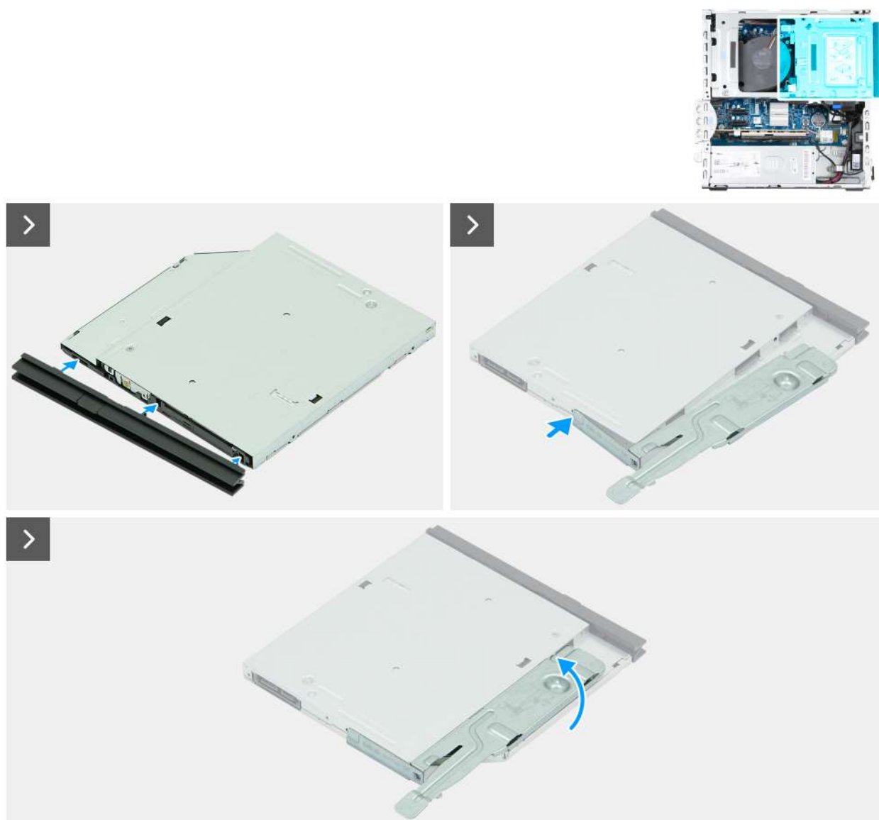
Figure 33. Installing the optical drive
