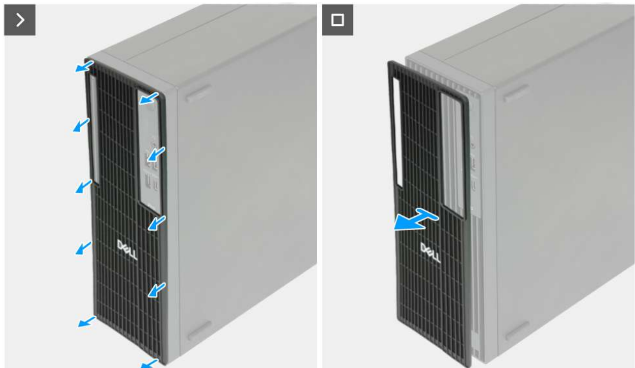
Figure 14. Removing the dust filter
