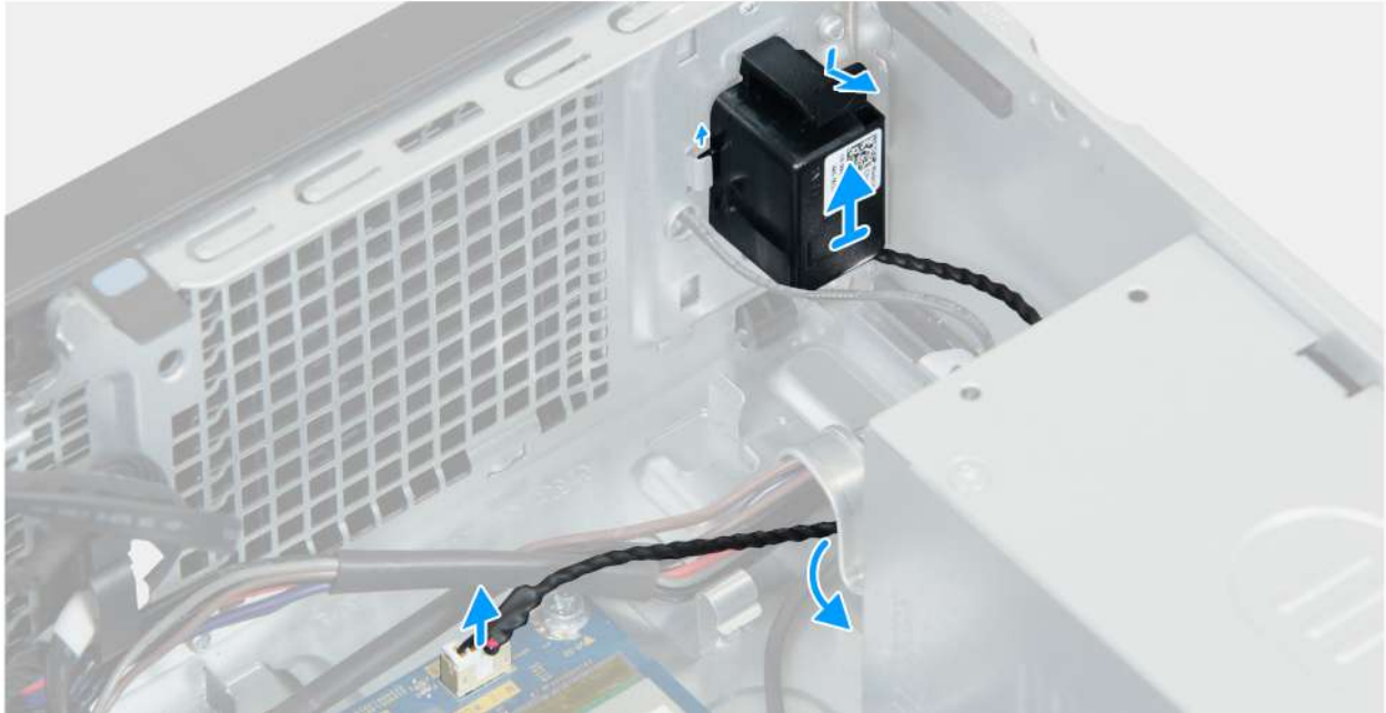
Figure 18. Removing the internal speaker
