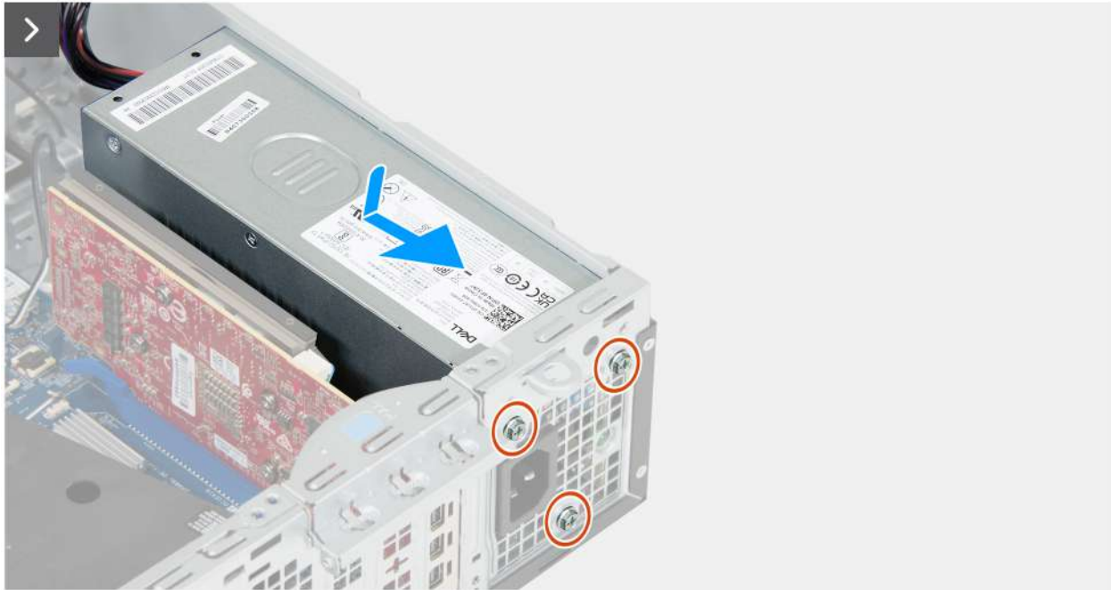
Figure 49. Installing the power-supply unit
