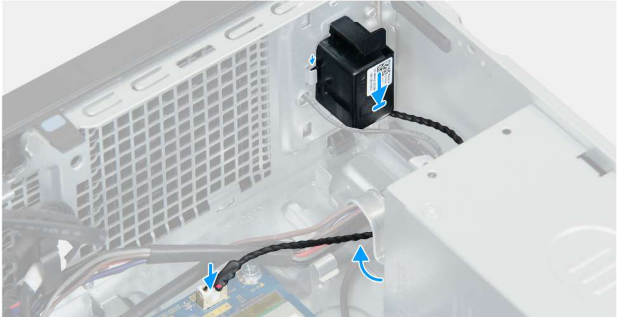
Figure 19. Installing the internal speaker
