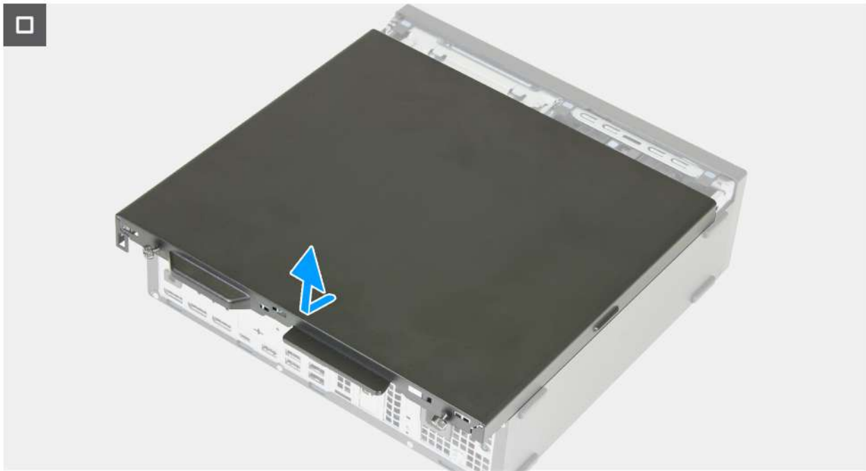
Figure 7. Removing the side cover
