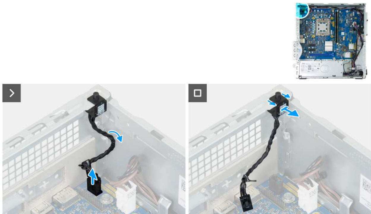
Figure 41. Removing the intrusion switch
