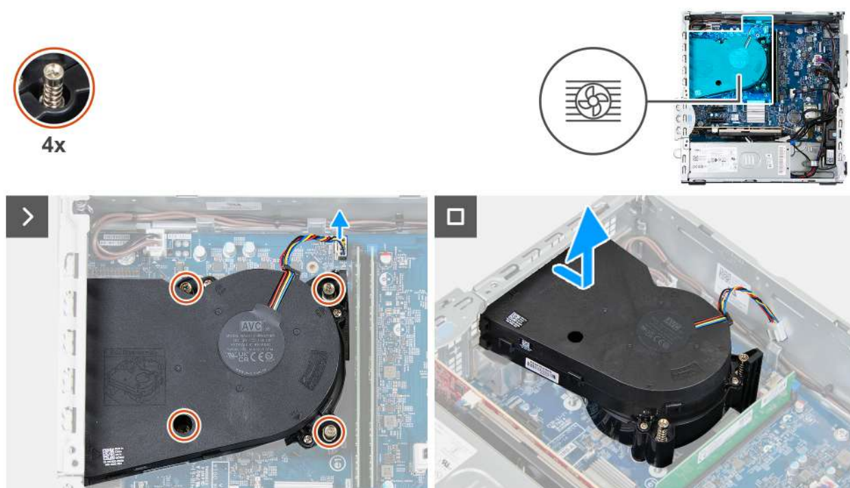
Figure 51. Removing the processor fan and heat-sink assembly
