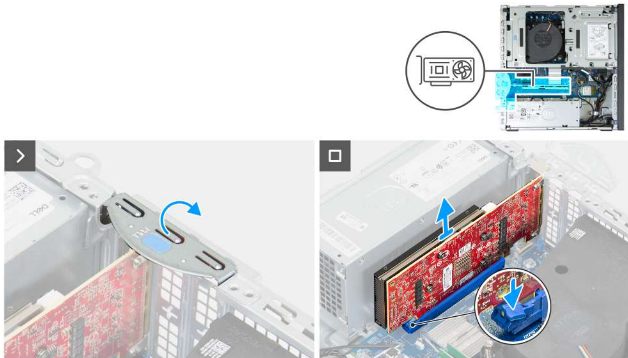
Figure 27. Removing the graphics card
