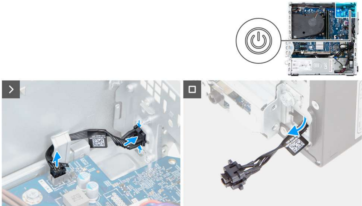
Figure 43. Removing the power button
