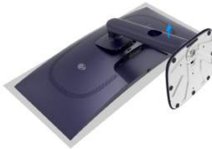
Figure 28. Removing the monitor stand
