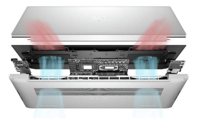
Advanced thermal design: The new XPS 17 delivers unprecedented performance (90W) in an incredibly thin (19.5,mm) form factor. A unique thermal design makes it possible to cool so much power in such a thin design.
