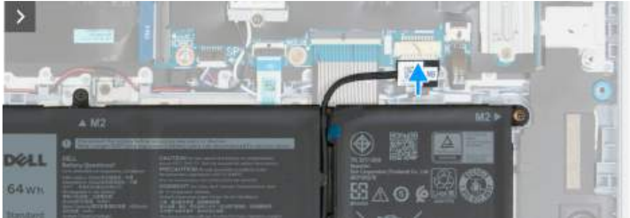
Figure 12. Connecting the battery cable
