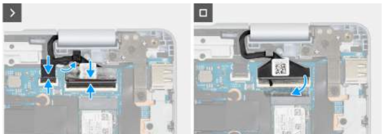
Figure 31. Installing the display assembly 2
