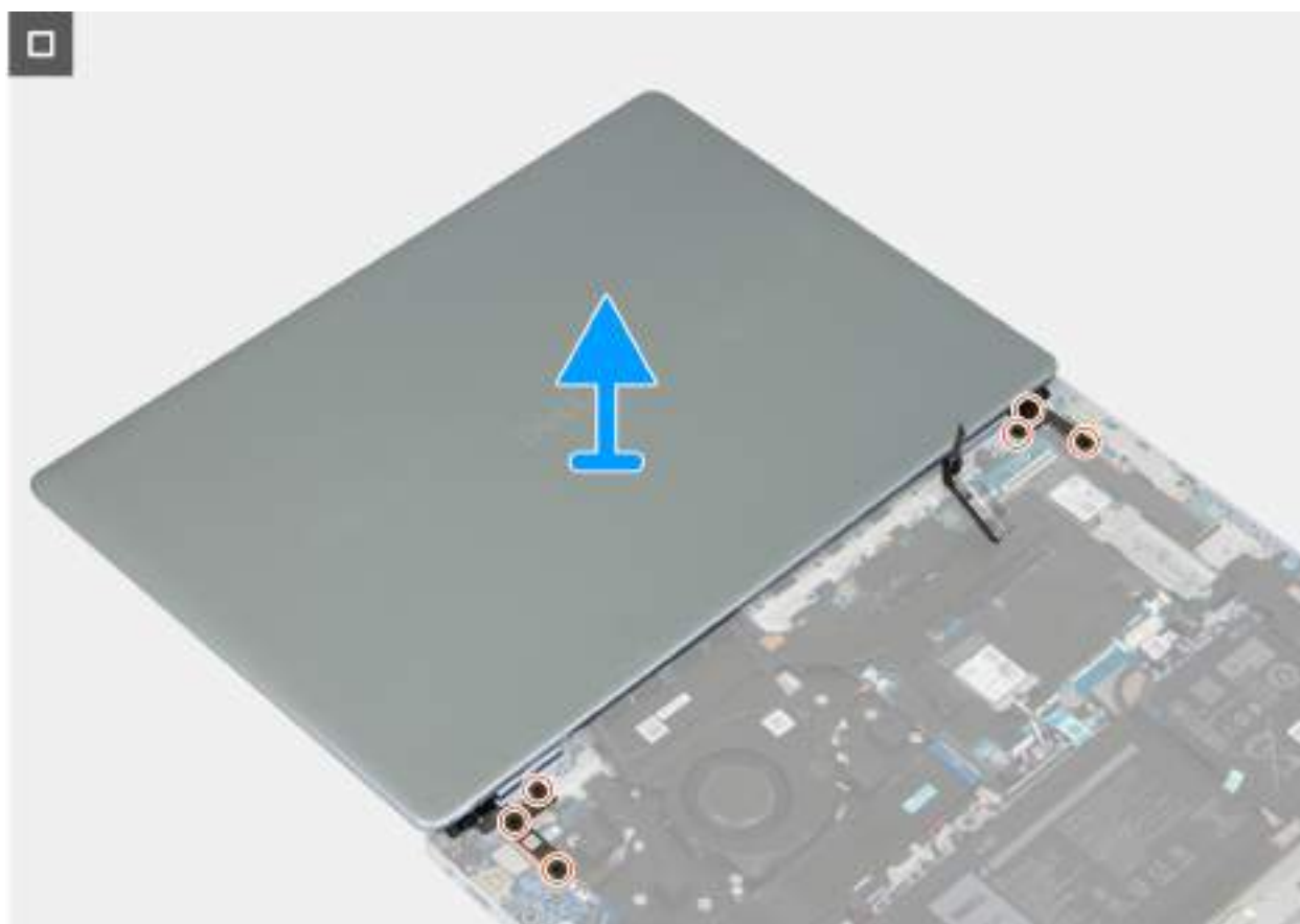
Figure 28. Removing the display assembly 2
