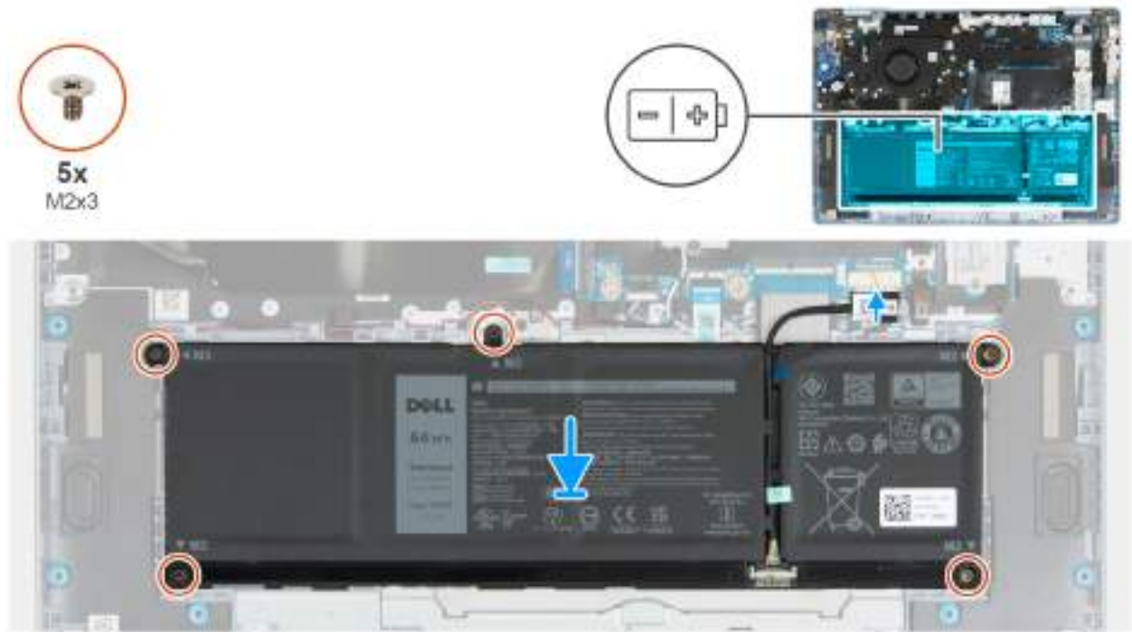
Figure 16. Installing the battery
