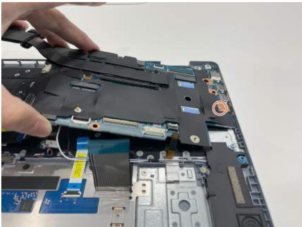
Figure 49. Installing the system board without damaging it
