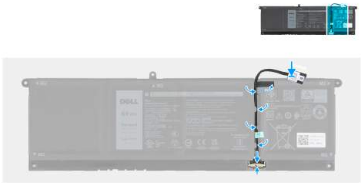
Figure 18. Installing the battery cable
