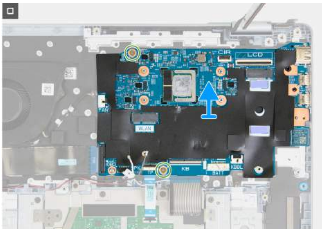
Figure 43. Removing the system board
