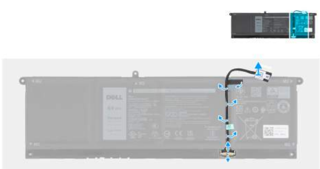
Figure 17. Removing the battery cable
