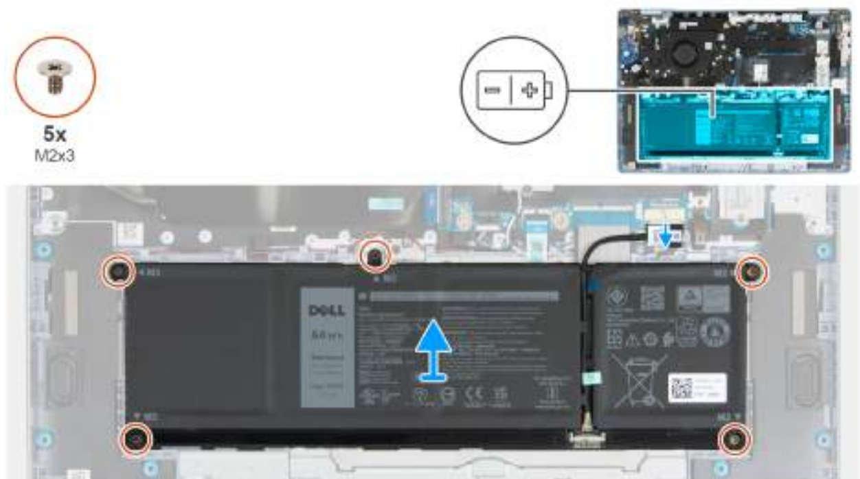
Figure 15. Removing the battery
