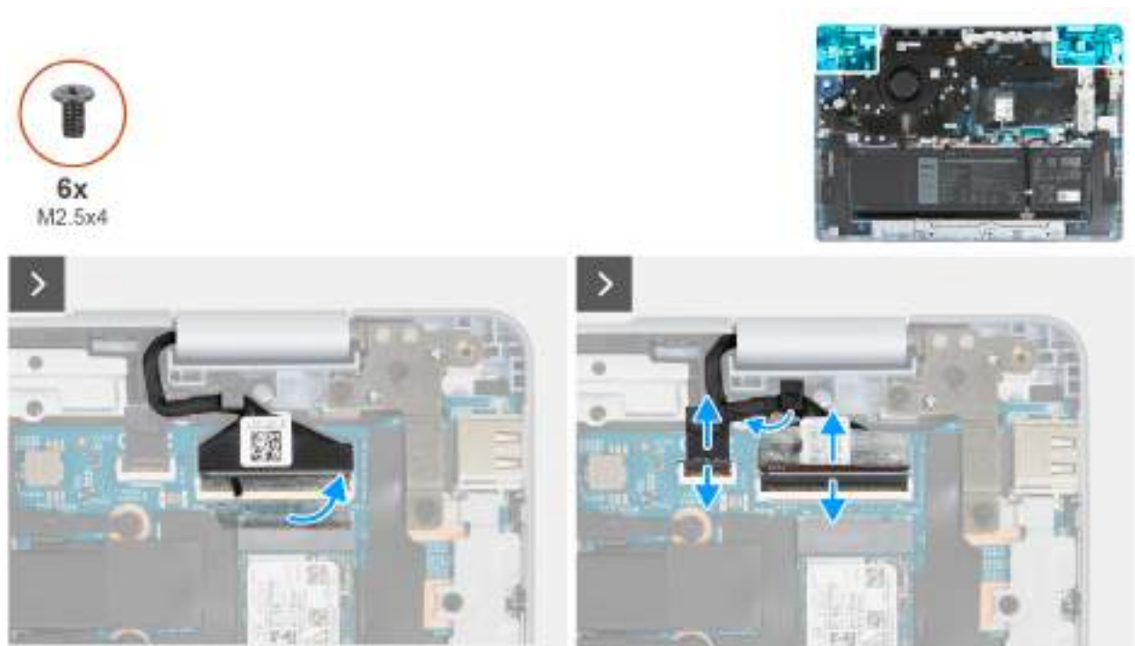
Figure 27. Removing the display assembly 1
