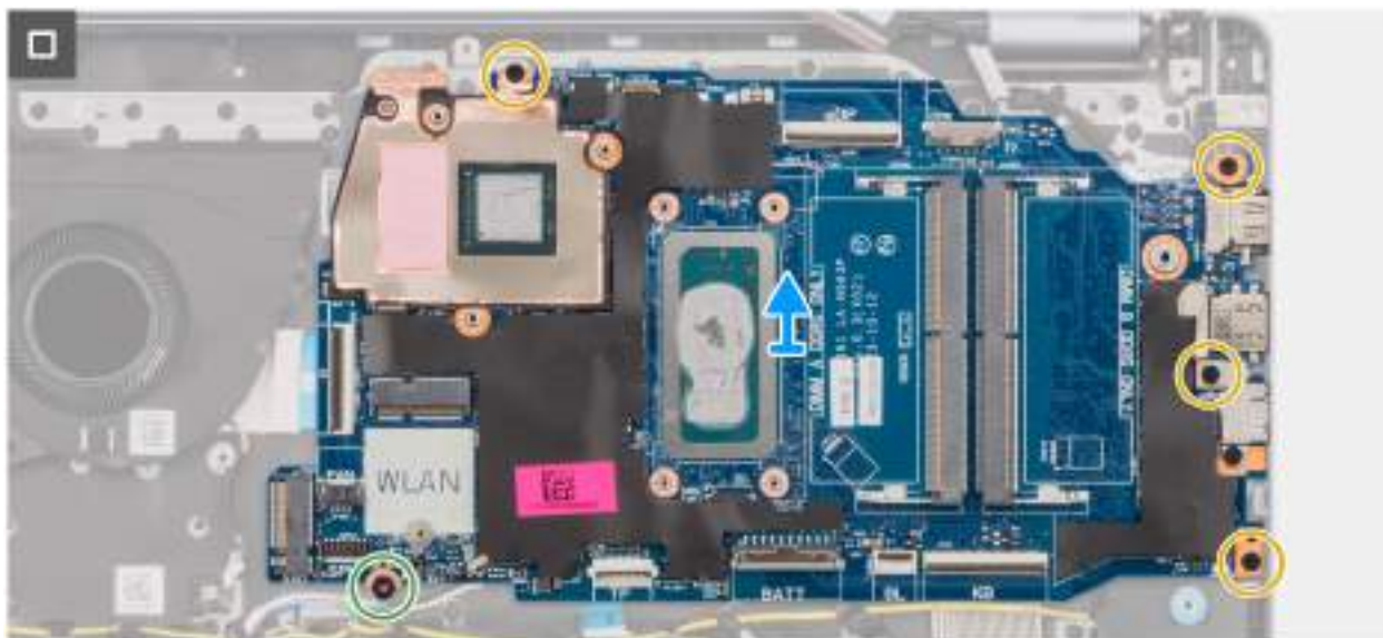
Obrázek 82. Removing the system board
