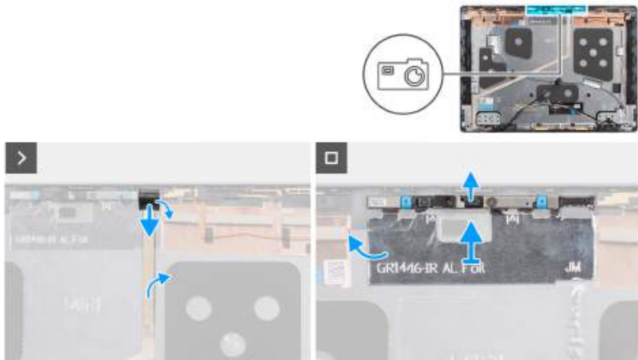
Figure 74. Removing the camera
