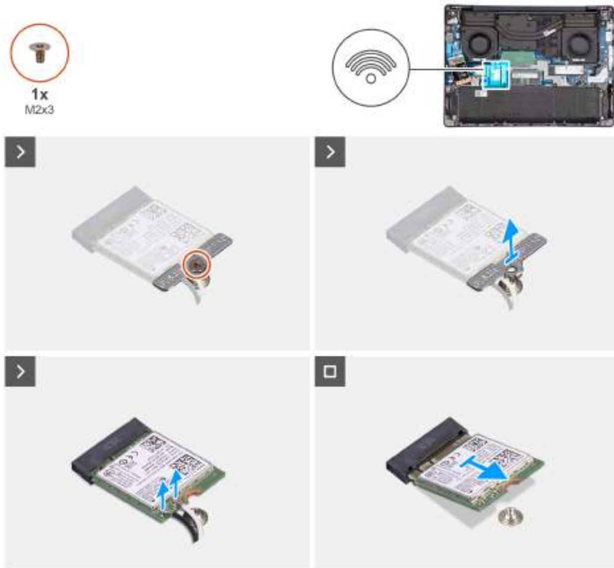
Figure 25. Removing the wireless card
