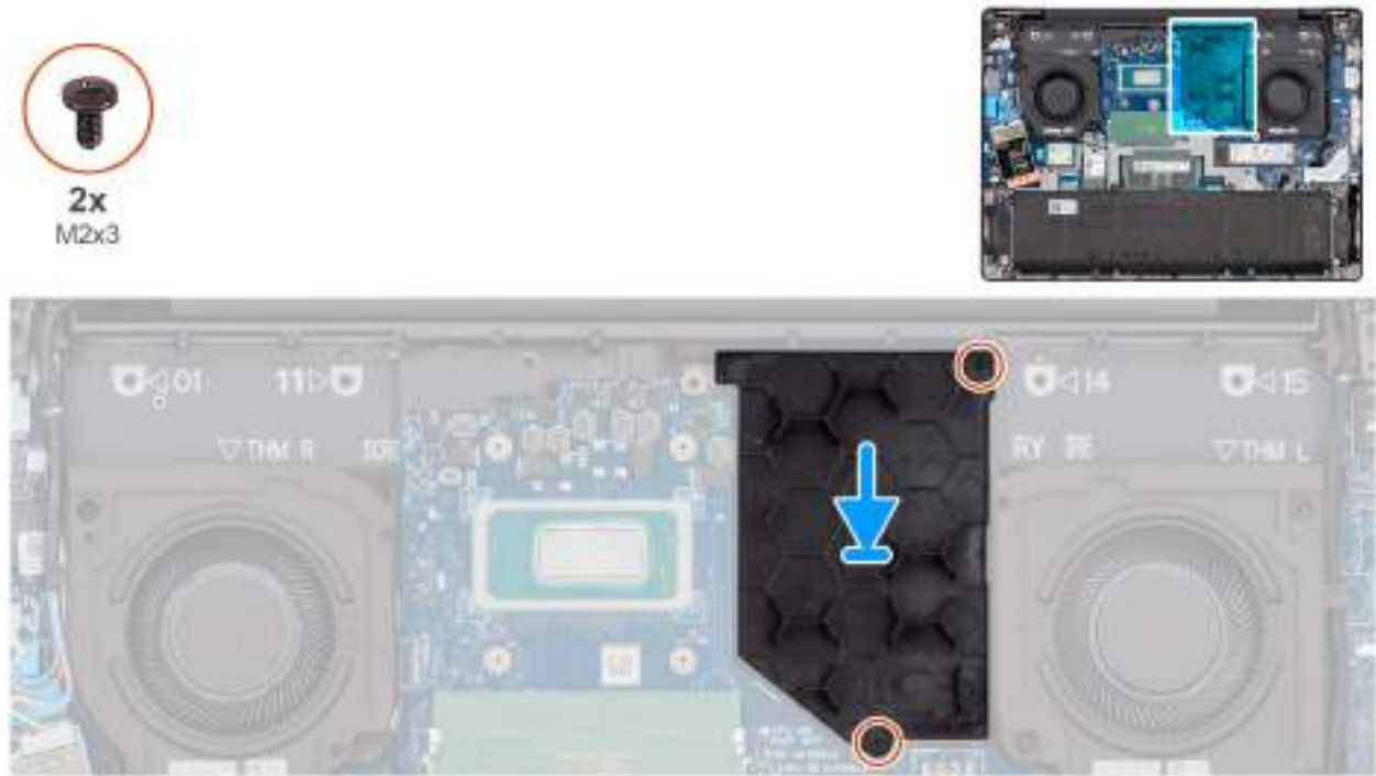
Figure 43. Installing the GPU filler
