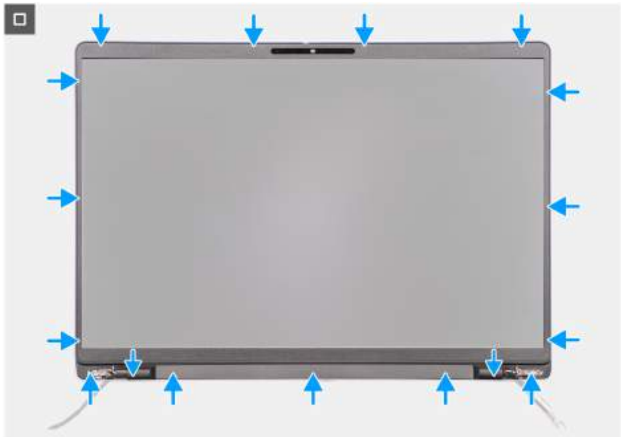
Figure 63. Installing the display bezel
