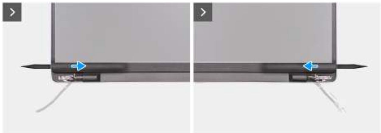
Figure 60. Removing the display bezel
