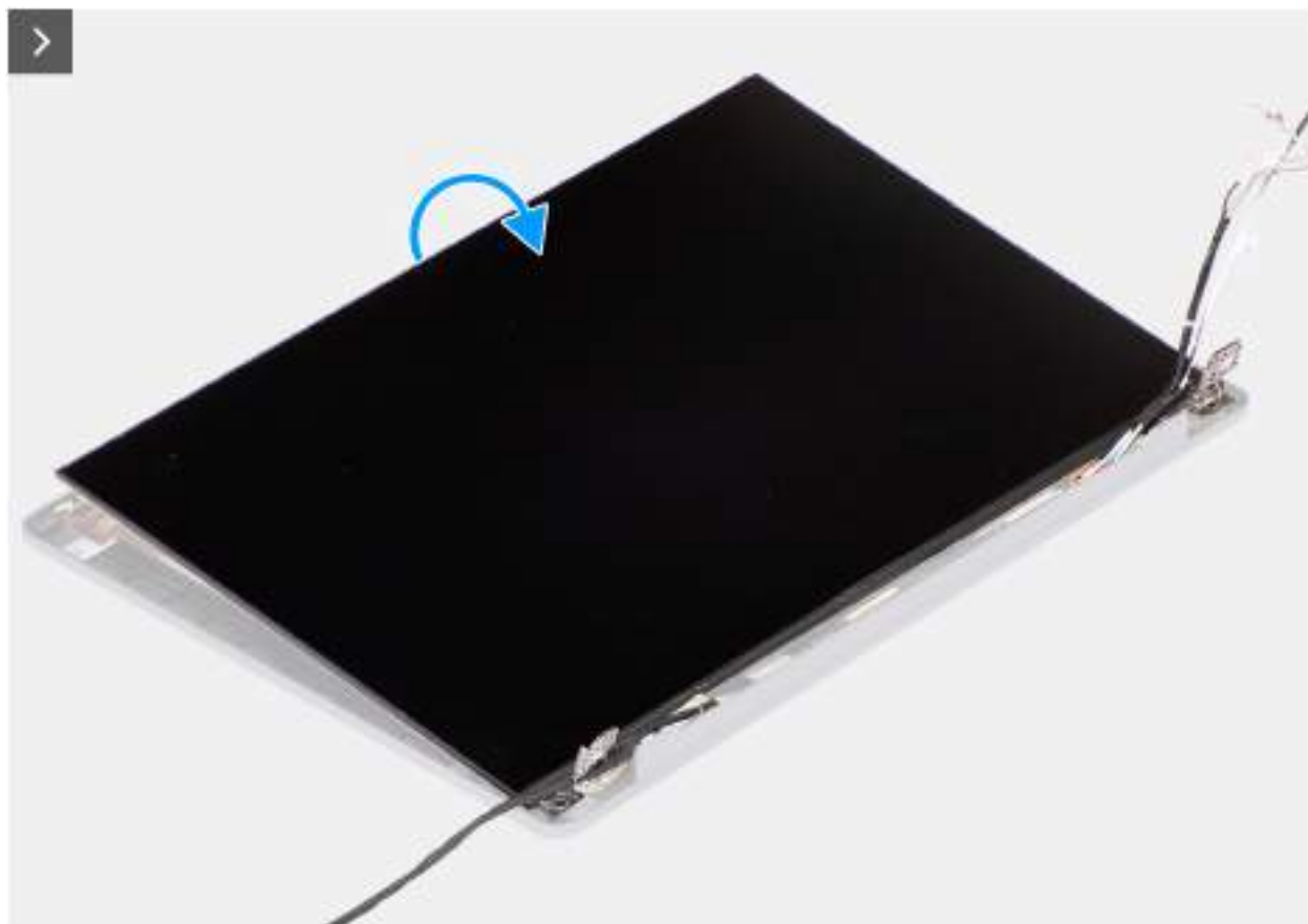
Figure 65. Removing the display panel
