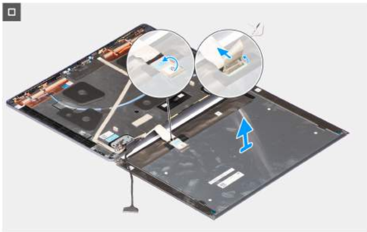
Figure 66. Removing the display panel
