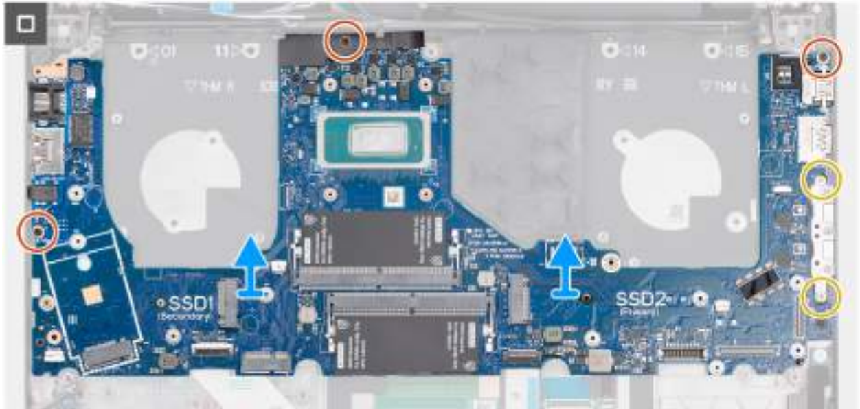
Figure 80. Removing the system board
