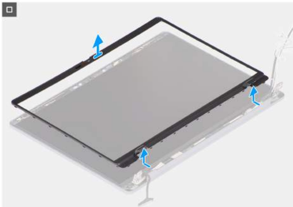
Figure 61. Removing the display bezel
