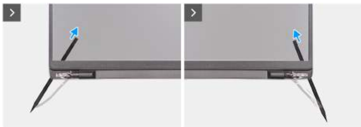
Figure 57. Removing the display bezel
