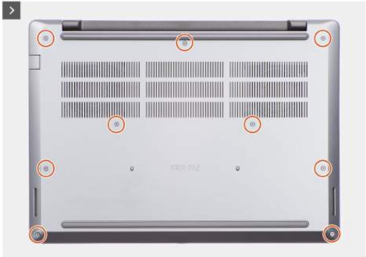
Figure 12. Removing the base cover
