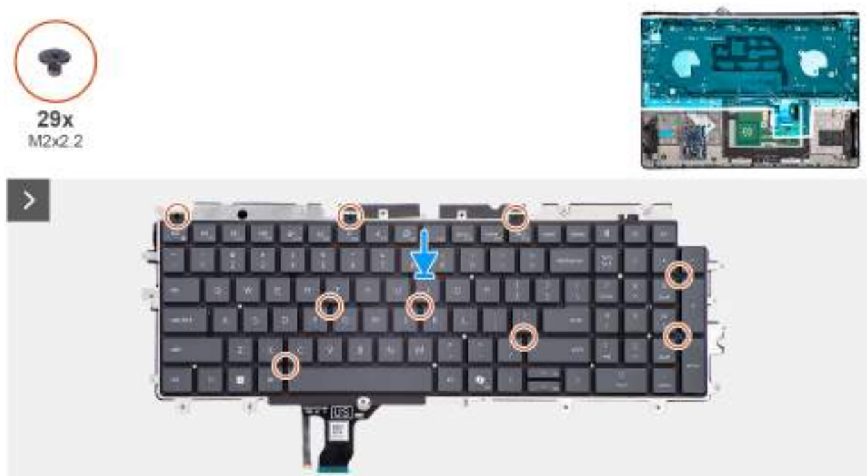
Figure 90. Installing the keyboard
