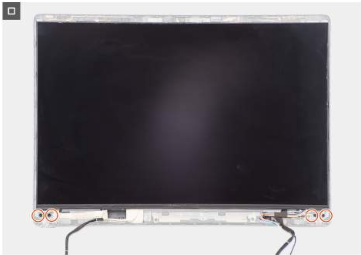
Figure 69. Installing the display panel
