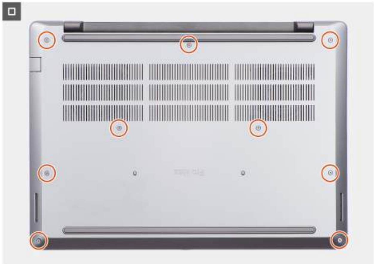
Figure 16. Installing the base cover
