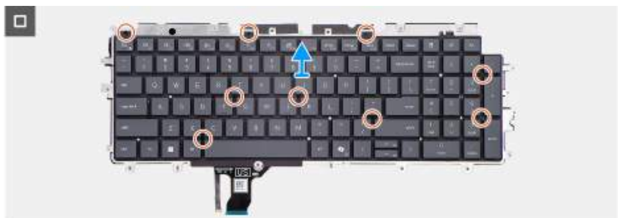
Figure 89. Removing the keyboard
