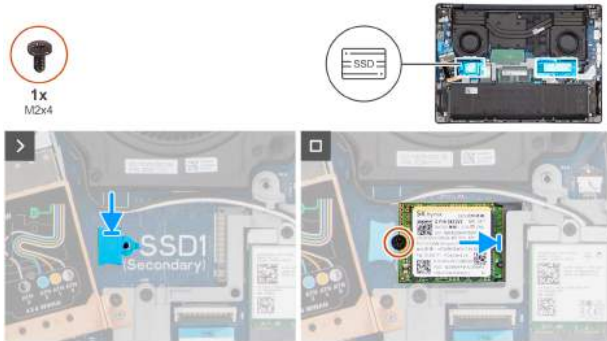
Figure 22. Installing the M.2 2230 solid state drive
