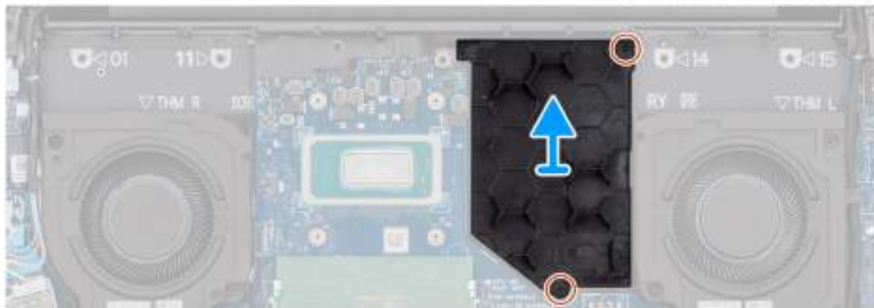
Figure 42. Removing the GPU filler
