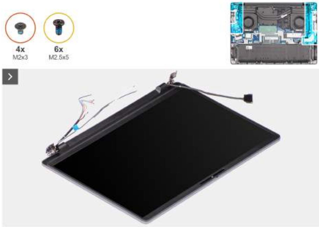
Figure 53. Installing the display assembly
