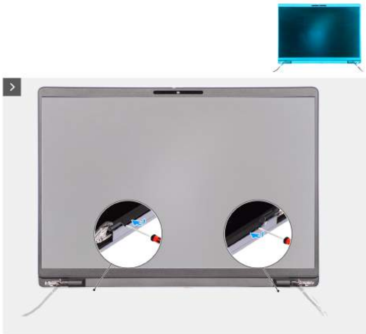
Figure 56. Removing the display bezel
