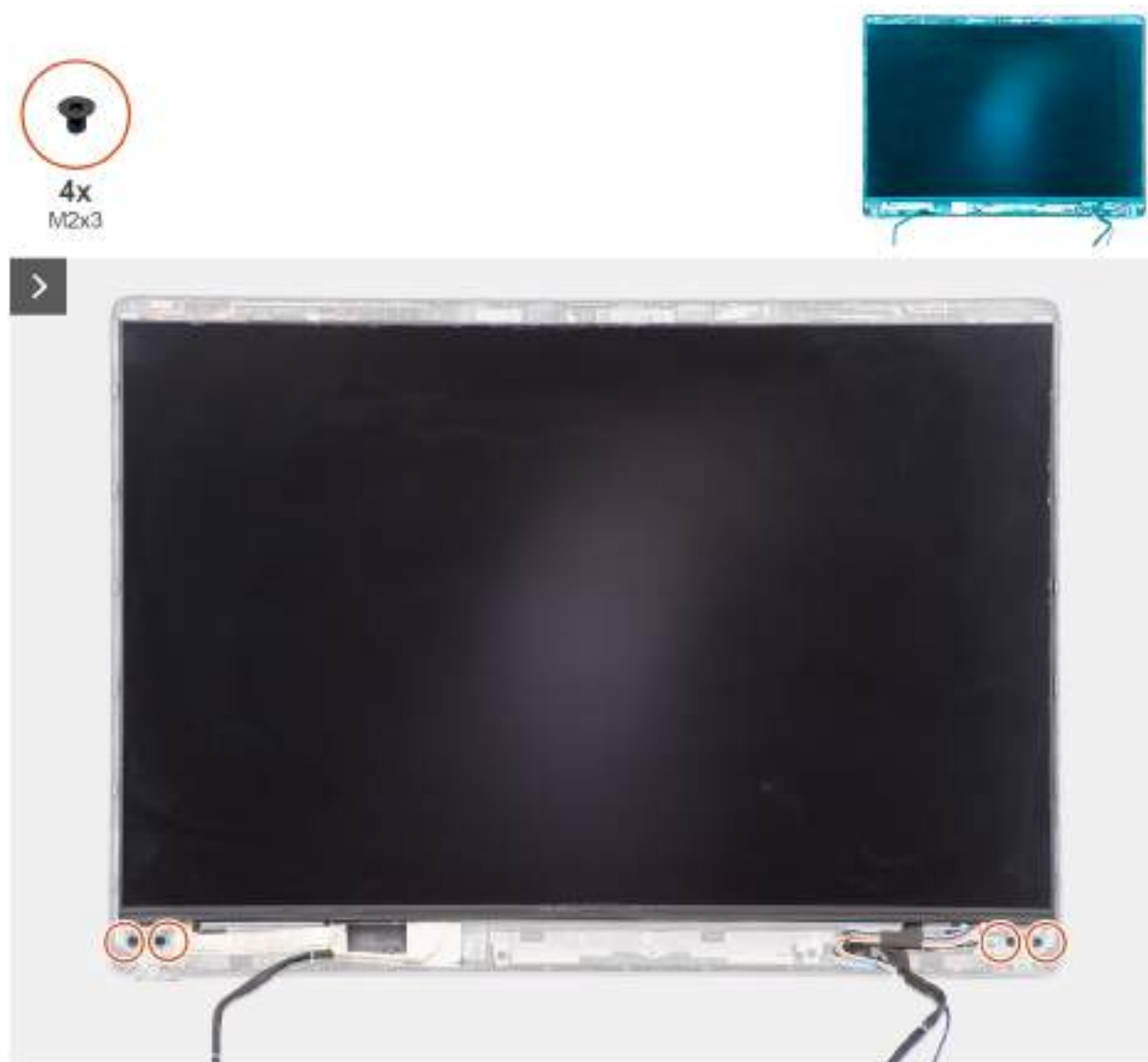
Figure 64. Removing the display panel
