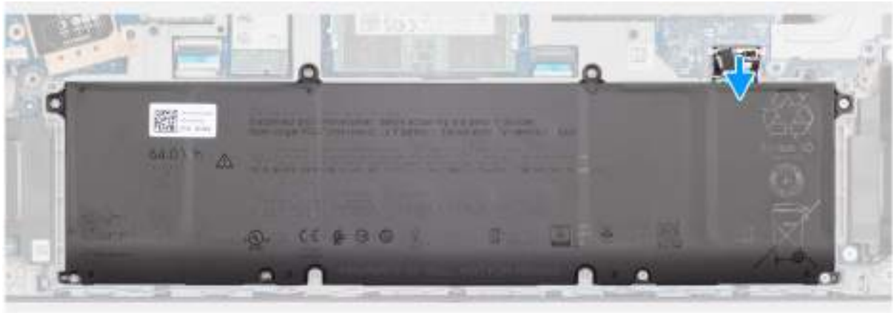
Figure 14. Removing the battery cable
