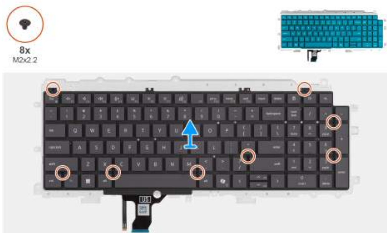
Obrázek 56. Removing the keyboard support plate
