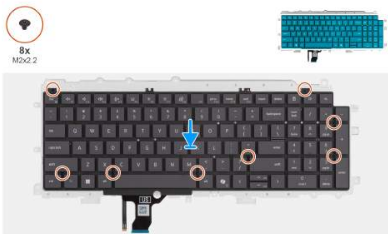
Obrázek 59. Installing the keyboard support plate
