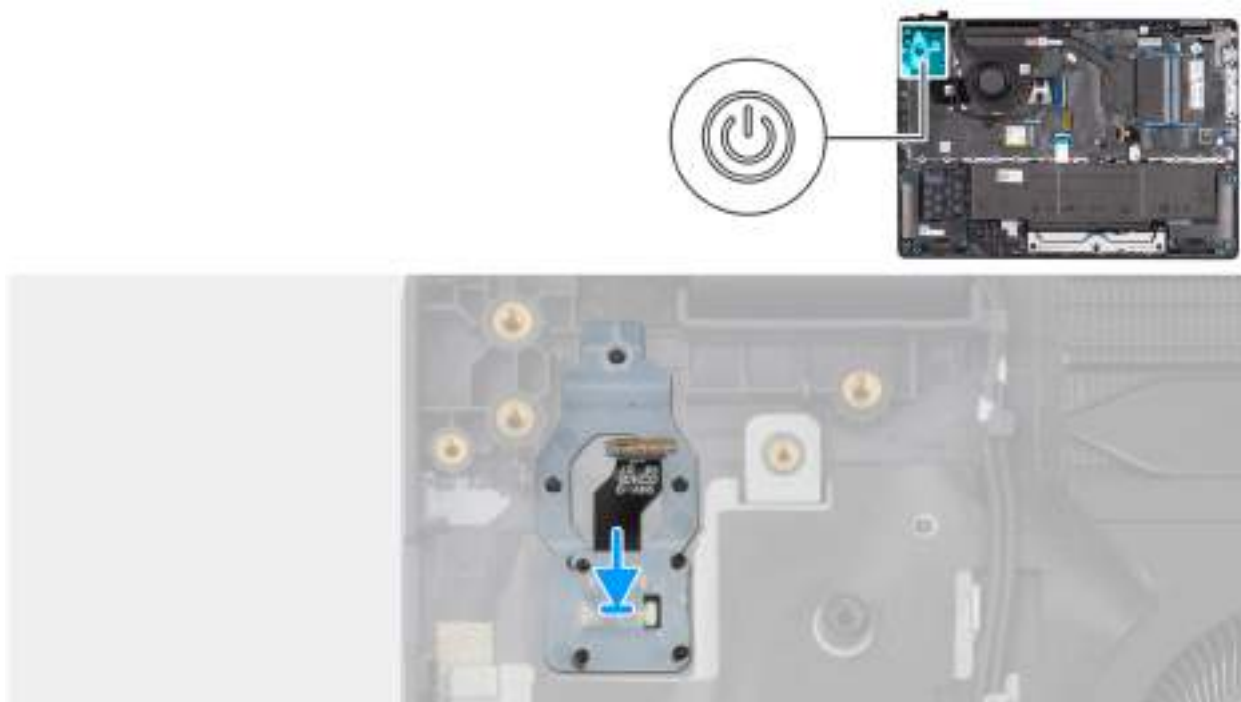
Obrázek 41. Installing the power button with a fingerprint reader
