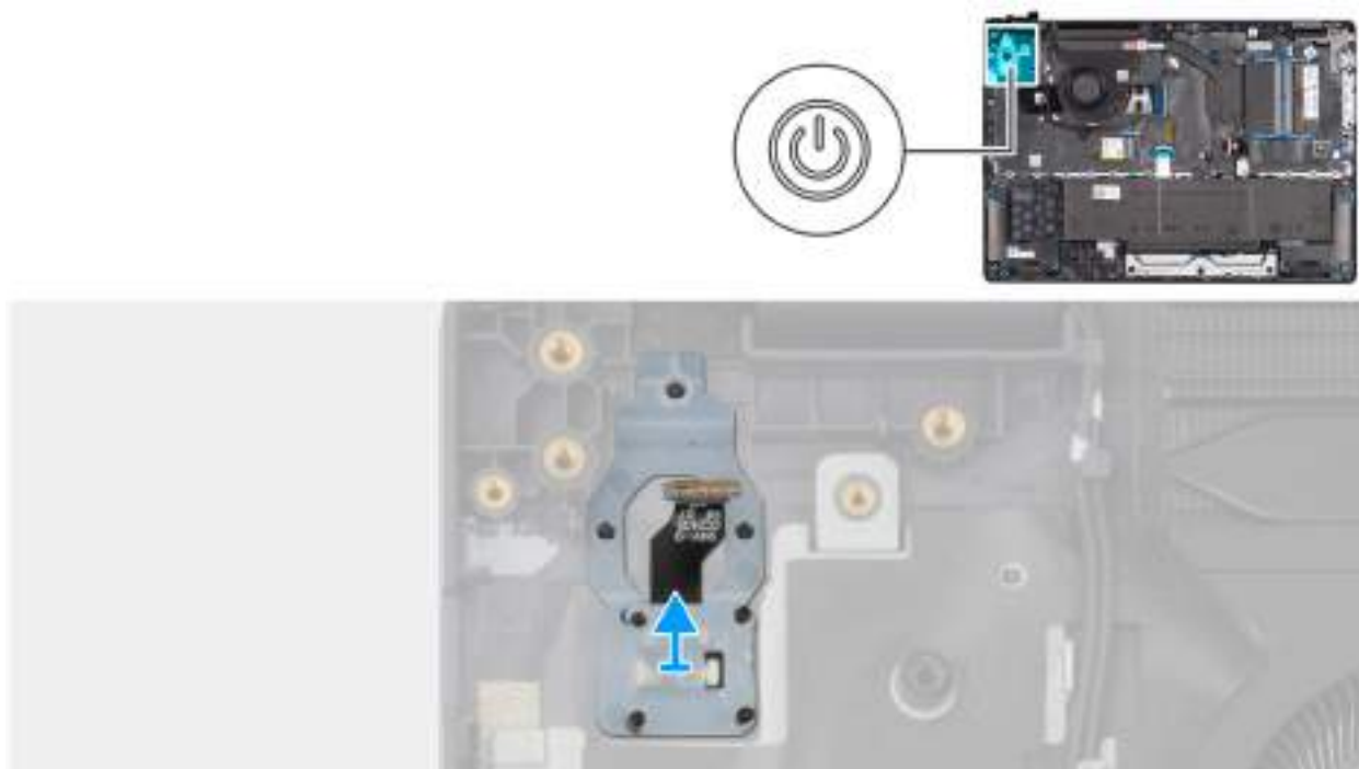
Obrázek 40. Removing the power button with fingerprint reader
