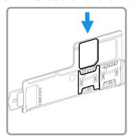
b. SIM 2 (model dependent): Slide the nano-SIM card into the card socket.
