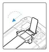
3. Unlock the battery. Press and hold down the small button on the battery latch, and then slide the latch toward the unlock icon. The battery will pop-up slightly on the edge when the latch is released.
