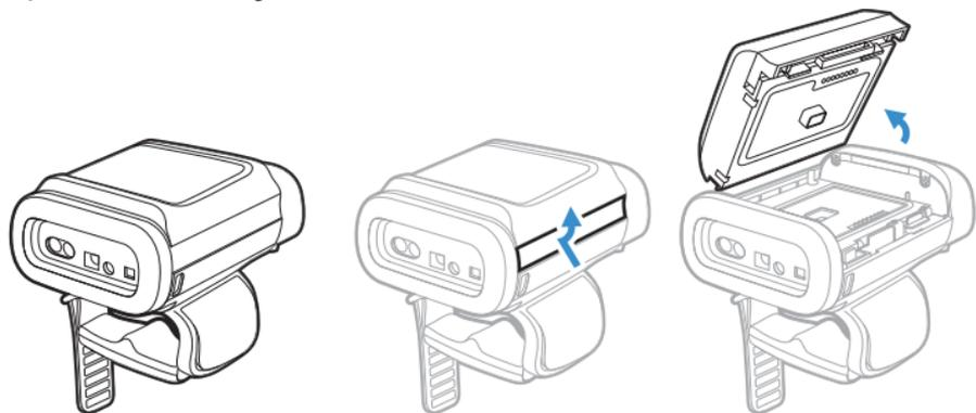
Replace the battery by snapping it in to the scanner.
