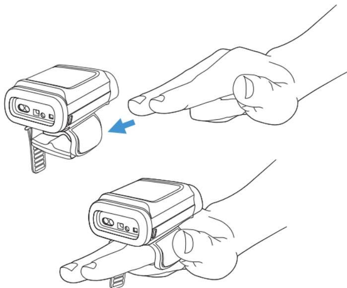
Pull the finger strap to secure it and tuck the excess strap length into the finger guide channel.
