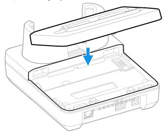
5. While holding the latch to the right, push the back of the cup into the base until it snaps in.
