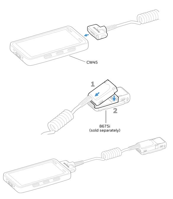
**Note:** If the connected CW45 is inserted into a charging base, communication with the ring scanner will be interrupted.
