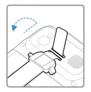
4. Unlock the battery cover. Press and hold down the small button on the battery latch and then slide the latch to the right.
