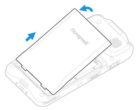
6. Use the tabs on the bottom of the battery to lift and remove it from the computer.
