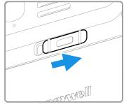
5. Lift the battery cover and remove it.
