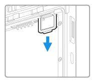
5. Place the nano-SIM card into the card holder tray with contacts facing down.
