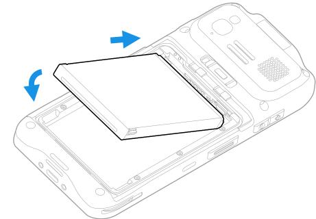
1. Insert the charged battery into the computer. The top of the battery must go in
