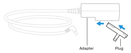
**Note:** The inside of the DC plug is negative; the outside is positive.
