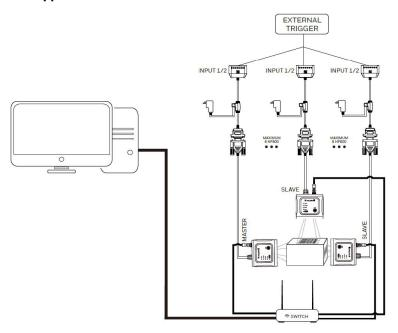
In Passthrough Mode, all the HF800 units can be triggered by one source or be triggered separately. The master will act as a repeater and transmit all of the data from the slave devices without processing through the master device's interface.
