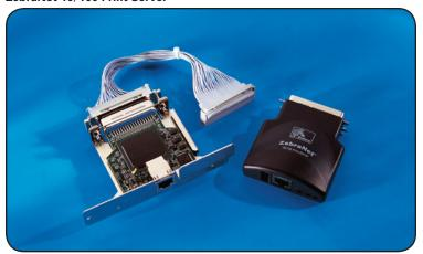
ZebraNet 10/100 Print Server is available in an internal or external version that provides a complete wired solution for 10Base-T, 100Base-TX, and fast Ethernet 10/100 autoswitching networks. When paired with the industrial-strength Zebra Xi, 105SL, S4M, Z4Mplus  $^{\text{TM}}$  / Z6Mplus  $^{\text{TM}}$  and ZM400/ZM600, RXi, RZ400/RZ600, RPAX printers with enhanced ECP parallel support, it offers greater data transmission speeds for faster throughput.
