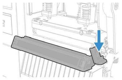
6. Move the inside toggle and outside toggle to the center of printhead.
