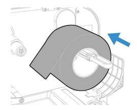
**Note:** Make sure you push the roll all the way against the inner wall of the printer.
