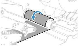
3. Lift the rewinder batch plate into place, lower the front arm, turn the printhead lift lever clockwise to close the printhead and click into place.
