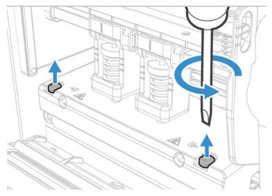
8. Turn the printhead lift leaver counter clockwise and put the printhead toward you to remove.
