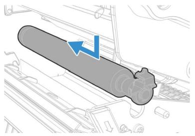
9. Lock the platen roller by rotating the latch counter clockwise.
