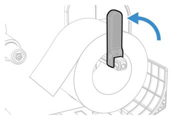
5. Turn the printhead lift lever counterclockwise to raise the printhead and lift the front arm.
