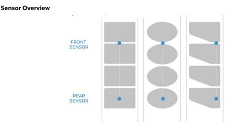
The sensor contains a blue LED that is strong enough to see through media. You can use the blue LED to help determine the proper location for the sensor.
