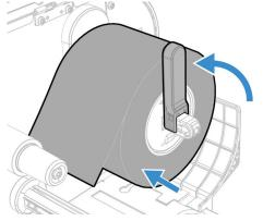
4. Lift the lever to open the peel-off module to route media to rewind hub.
